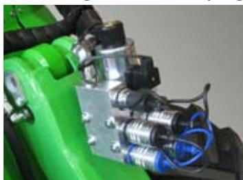
Two auxiliary hydraulics outlets in the front
